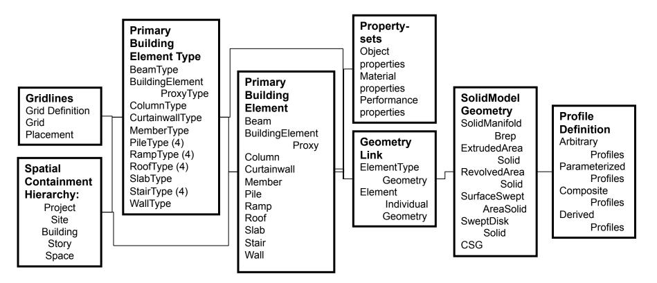
A Model View is a directed sequence of Elements that incrementally map to the existing IFC structure
