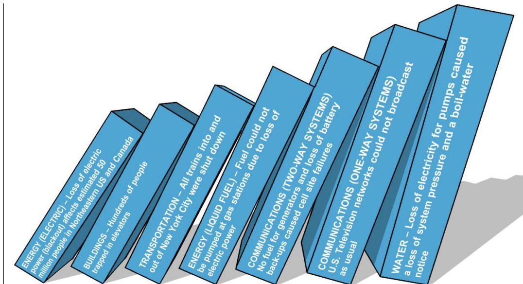
Figure 11-4: External dependence cascading failure in the 2003 Northeast Blackout
