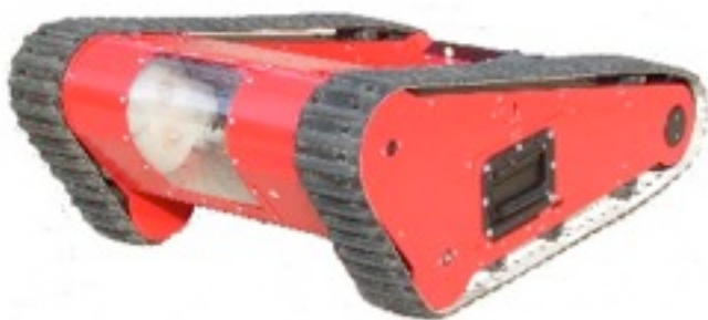
A common robot mobility platform for the league, the Mesa Element, is $12K USD with serial and USARsim interfaces ( www.mesa-robotics.com )
