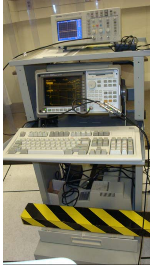
Figure 4d: Oscilloscope and Dynamic Signal Analyzer Measuring Frequency Response
