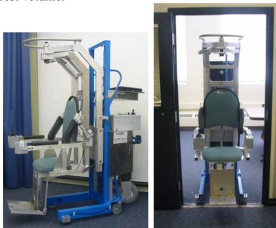
**Figure 2 – Photographs of the HLPR Chair in the mobility configuration showing the side view (left) and front view relative to a typical doorway (right).**
