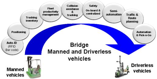
Figure 1 – Drawing showing sensors, logistical aspects and tasks needed to bridge between manned and driverless vehicles
