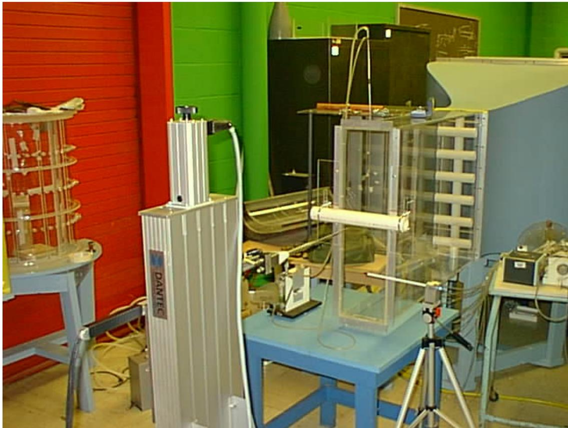
Figure 8-85. Low-speed, High-turbulence, Open Jet USNA Wind Tunnel.
