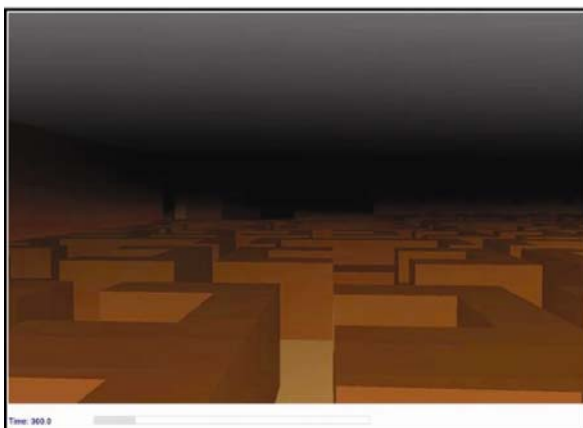
Figure K- 21. Smoke progression inside the west showroom between 240 s to 390 s (7:14:53p.m. to 7:17:23 p.m.).
