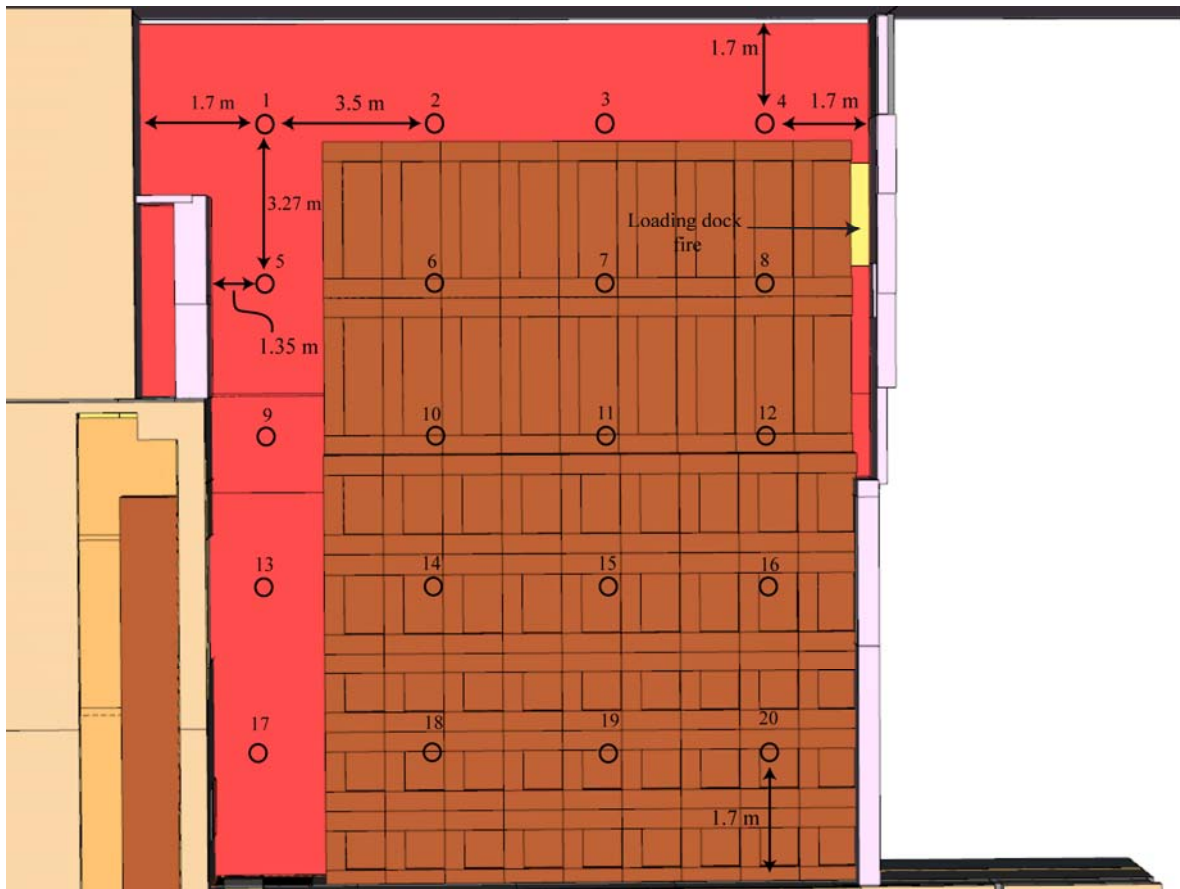
Figure K-41. Simulated sprinkler layout inside the enclosed loading dock.
