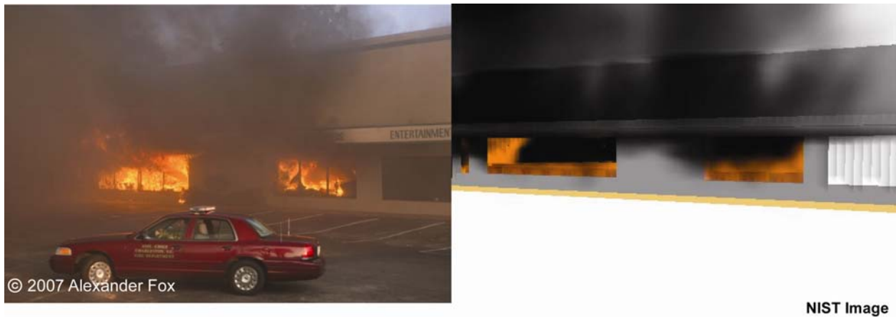
Figure K-26. Comparison between photo and rendered image from the simulation at 1686 s (7:38:59 p.m.). The view is of the front of the main showroom. Photo used with permission of Alexander Fox.
