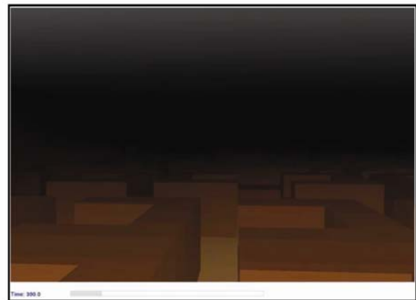
Figure K- 21. Smoke progression inside the west showroom between 240 s to 390 s (7:14:53p.m. to 7:17:23 p.m.).
