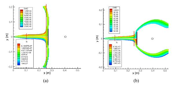
Figure 4. Predicted water-mist Sauter mean diameter (SMD) and number density (N) profiles evolving around an obstacle with (a) no coflow and (b) a 5 m/s coflow.
