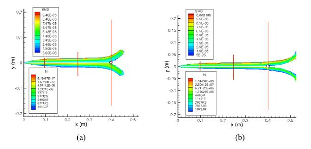
Figure 3. Predicted water-mist Sauter mean diameter (SMD) and number density (N) profiles with (a) no coflow and (b) a 5 m/s coflow.
