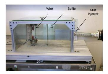
Figure 1. Experimental apparatus for electrical fire suppression tests based on the Space Shuttle mid-deck locker.
