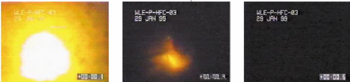
**Figure 2-67. Time Sequence of Dry Bay Compartment Fire Suppression by Inert Gas Generators, Complete Suppression within 600 ms.**<sup>139</sup>
