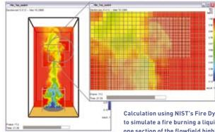
Calculation using NIST's Fire Dynamics Simulator (FDS) software to simulate a fire burning a liquid hydrocarbon fuel. A blow-up of one section of the flowfield highlights computational techniques being developed to enable more accurate calculations.
