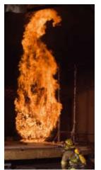
BFRL conducts experiments of burning trees in order to validate predictions of heat fluxes and heat release from simulated trees using the Wildland-Urban Interface Fire Dynamics Simulator (WFDS). WFDS is a physics based numerical modeling approach which includes all modes of heat transfer (convection, conduction. and radiation).
