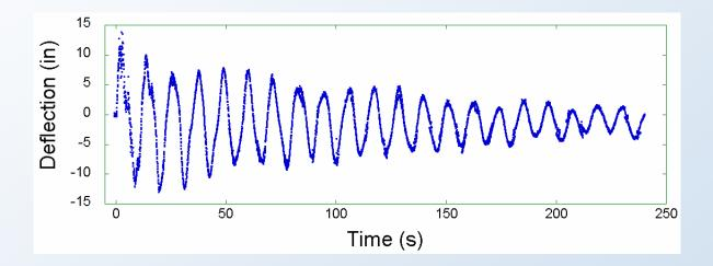
The WTC towers displayed significant reserve capacity, vibrating immediately following impact with amplitudes that were about half the amplitudes for design wind conditions expected by the building designers and an oscillation period nearly equal to that measured for the undamaged building.
