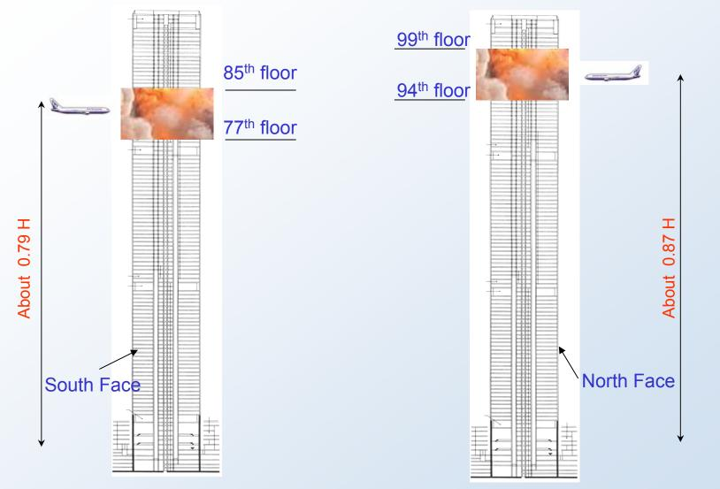
South tower: Hit at 9:02:59 AM Collapsed after 56 minutes
