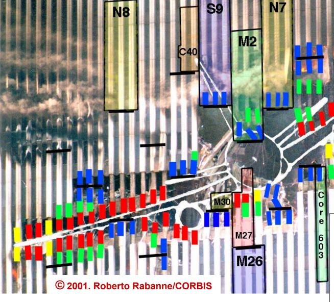
Broken Bolt Connection Column or Spandrel Cut Longitudinal Weld Failure Unknown Panel Junction
