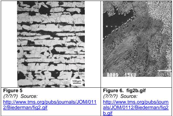
The microstructure of unaffected A36 steel: (Figure Error! Reference source not found.) white-ferrite, dark-pearlite and (Figure Error! Reference source not found.) pearlite region. Pearlite forms in bands due to manganese segregation and prior hot working.
