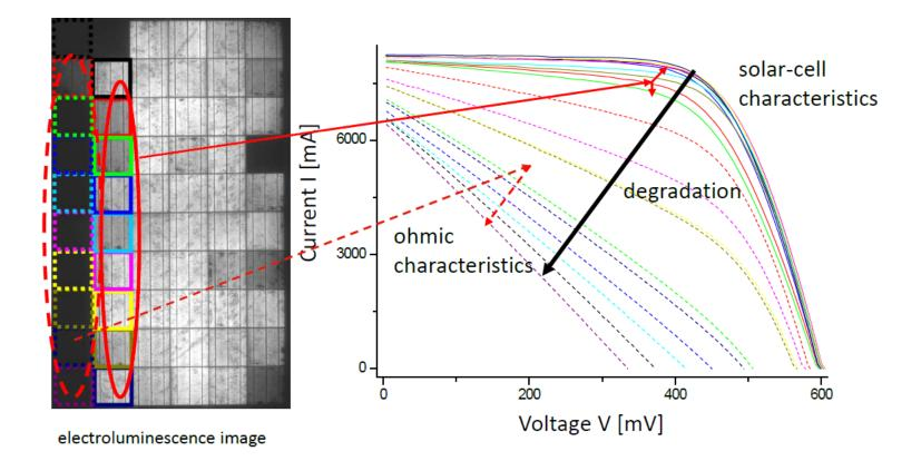
PID-s  $\rightarrow$  Potential induced degradation by shunting of solar cell
