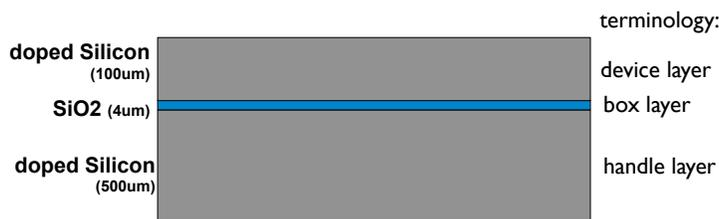
Figure 8.37: Figure showing a typical silicon on oxide (SOI) wafer in cross section. Note that the illustration is not drawn to scale.
