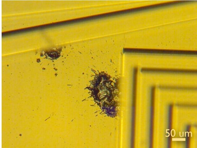
Figure 8.23: The micrograph shows evidence of breakdown on a SOI structures due to charging in the Plasma Ops III oxide etcher.
