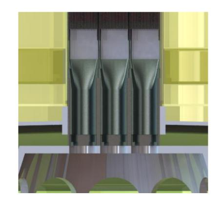
Fig. 2. 18-Plate fuel assembly in MNR.
