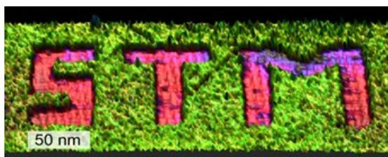
**Figure 1.** STM image of combined nanolithographic, covalent and non-covalent molecular functionalization of graphite
