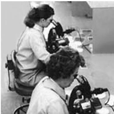
FIGURE 1. Wafer Inspection in the nineteen-sixties at Fairchild Semiconductor. Note that clean room attire was limited to a smock. Hair nets would be added by the seventies.
