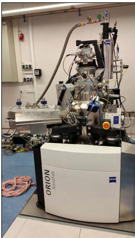
**FIGURE 1.** 3<sup>rd</sup> generation prototype of a GFIS based Microscope & SIMS combined instrument.
