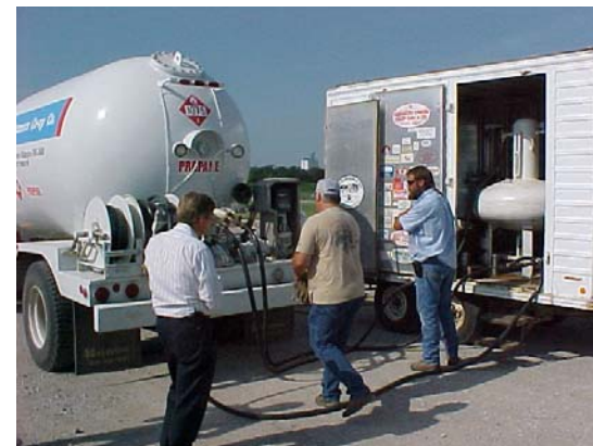
state field standards: testing an LP gas meter
