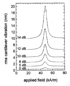
FIG. 4. Cantilever vibration vs applied field for a 30 nm Co film at different relative input microwave power levels.
