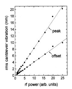
FIG. 5. Lorentzian peak and offset cantilever vibration vs input power for a 30 nm Co film (derived from the data in Fig. 4).
