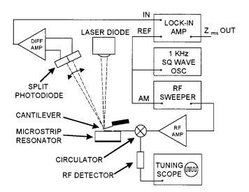
FIG. 2. Detection electronics for FMR thermal absorption spectroscopy.
