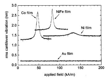
FIG. 3. Cantilever vibration vs applied field showing microwave absorption in Co, NiFe, Ni, and Au thin film samples.
