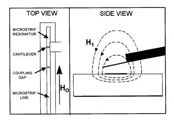
FIG. 1. Top view and side view of the experimental configuration for FMR thermal absorption spectroscopy. Note that the magnetic film samples are deposited on the upper side of the cantilever.
