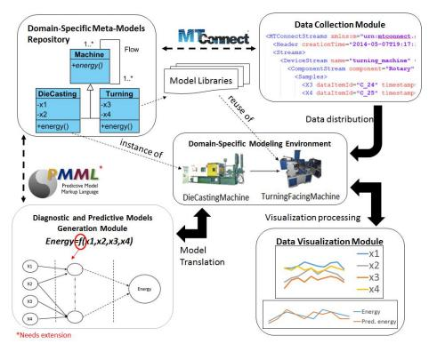
Fig. 1. Overview of the domain-specific framework for predictive analytics in manufacturing
