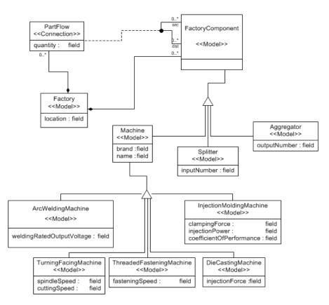
Fig. 3. Example meta-model for manufacturing production
