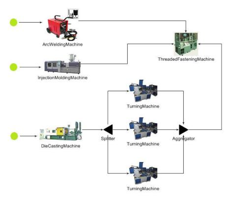
Fig. 2. Example of a production chain
