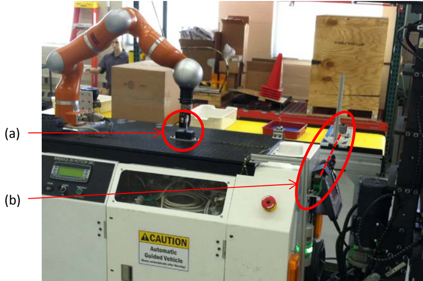
Figure 2: Robot onboard an AGV with low level safety control verification (a) stow switch used for Test 1 and (b) beam break switch used for Test 2.
