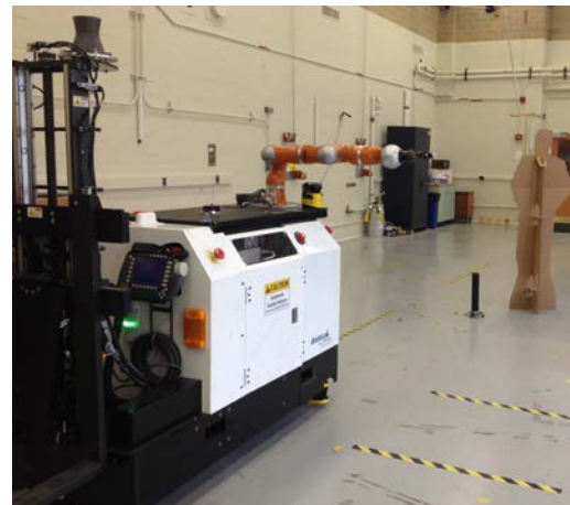
Figure 1 – Graphic (left) and photo (right) of a robot mounted onboard and collaborating with an AGV with a forklift for safe operation.
