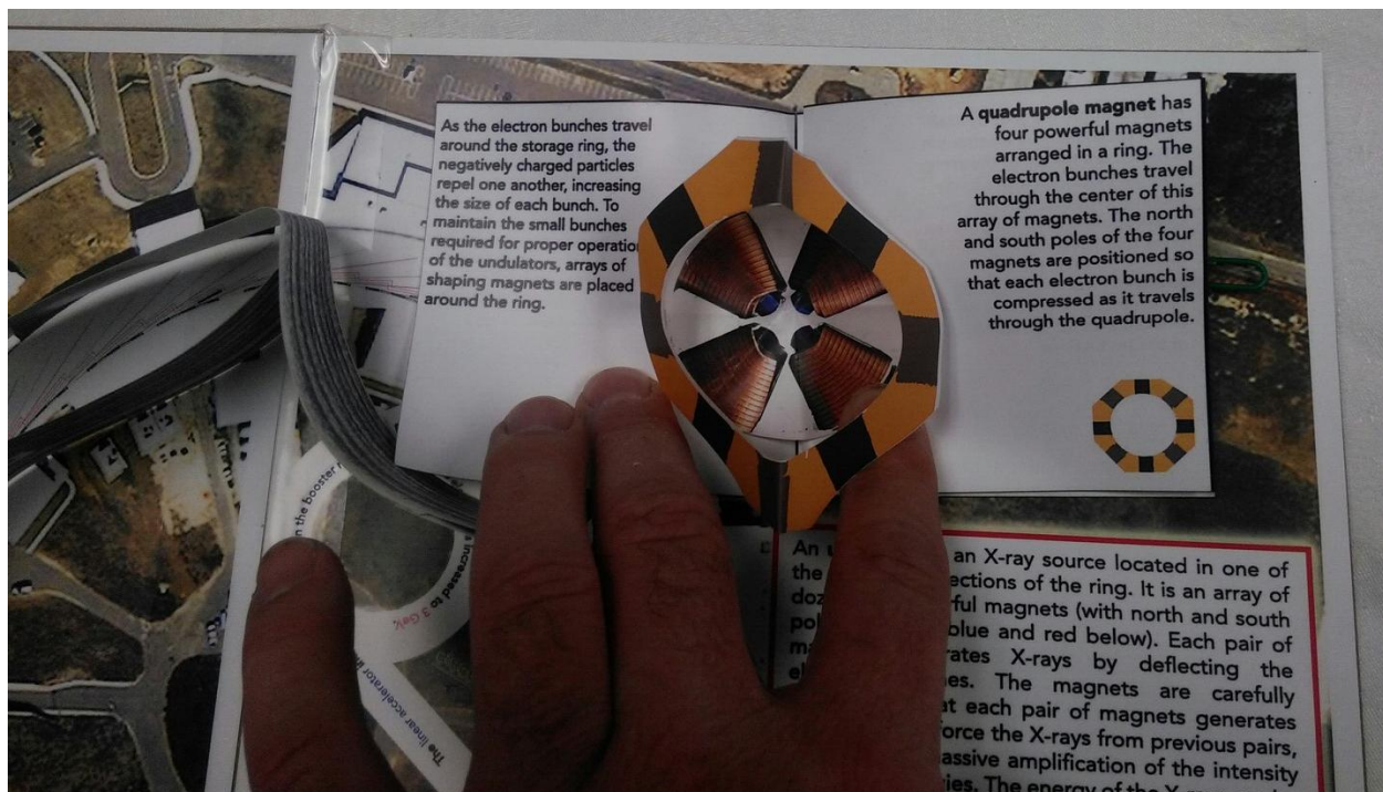
In the upper right corner is a booklet explaining how the quadrupole and sextupole magnets work to shape the electron beam, maintaining the small size required for the world-leading performance of NSLS-II.
