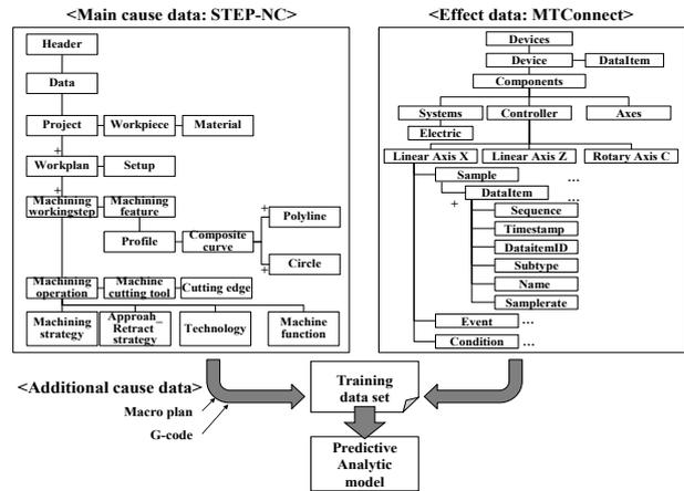
Fig. 1. Structures of cause-effect data and problem definition.
