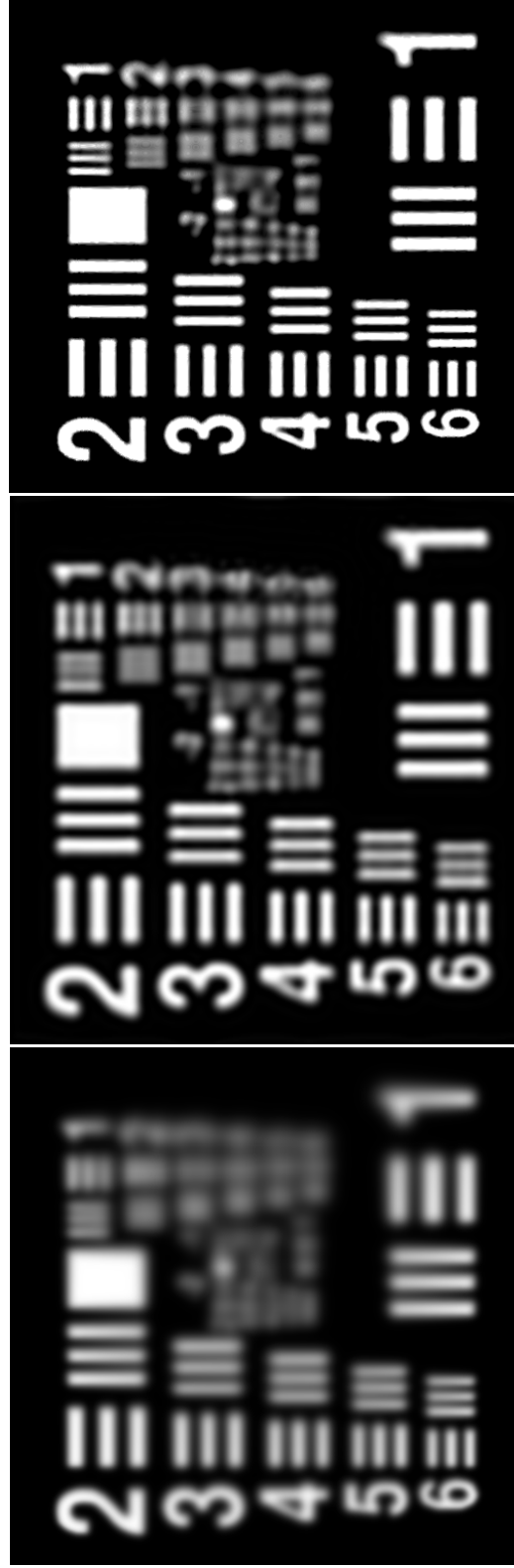
FIG. 8.3. In 512 \times 512 resolution chart image, stabilized backward time-marching in Eq. (3.3), with \epsilon = 3.5 \times 10^{-4} , p = 2.5 , competently recovers vertical sequence of numbers near image right edge in relatively little computing time, while the Van Cittert iteration is computationally impractical on large problems.
