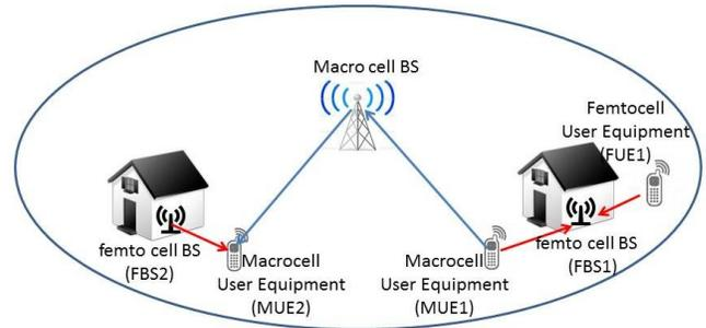
Fig. 2. Inter-cell interference between macro and femtocells
