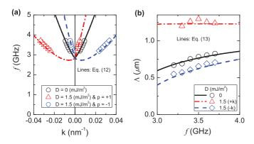
FIG. 4. (Color online) Asymmetric spin-wave propagation induced by an interfacial DM interaction in the small-*k* limit. (a) Dispersion relation. (b) Attenuation length  $\Lambda$  as a function of the frequency *f*. Symbols and lines correspond to numerical and analytic results, respectively.
