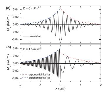
FIG. 2. (Color online) Snapshot images of spin-wave distribution along the x axis for (a) D = 0 mJ/m<sup>2</sup> and (b) D = 1.5 mJ/m<sup>2</sup>. The spin-wave frequency f is 11 GHz.
