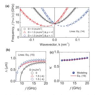
FIG. 3. (Color online) Asymmetric spin-wave propagation induced by an interfacial DM interaction in the large-*k* limit. (a) Dispersion relation. (b) Attenuation length  $\Lambda$  as a function of the frequency *f*. (c) Amplitude ratio  $\kappa$  as a function of *f*. Symbols and lines correspond to numerical and analytic results, respectively.
