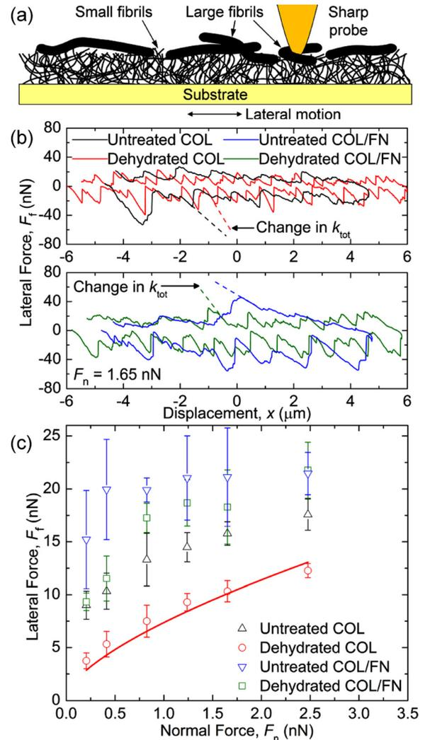
FIG. 3. (a) Schematic diagram of a sharp probe in contact with a COL film.  $F_f$  as a function of (b)  $x$  and (c)  $F_n$  for the untreated and dehydrated COL films with and without FN. In (b), there are a number of stick-slip events with a single instability, the slope of which are  $k_{\text{tot}}$ . In (c),  $F_f$  varies *sublinearly* with  $F_n$  for all films; the solid line represents a fit to the dehydrated COL data using the JKR model, with  $\tau$  as the fitting parameter.
