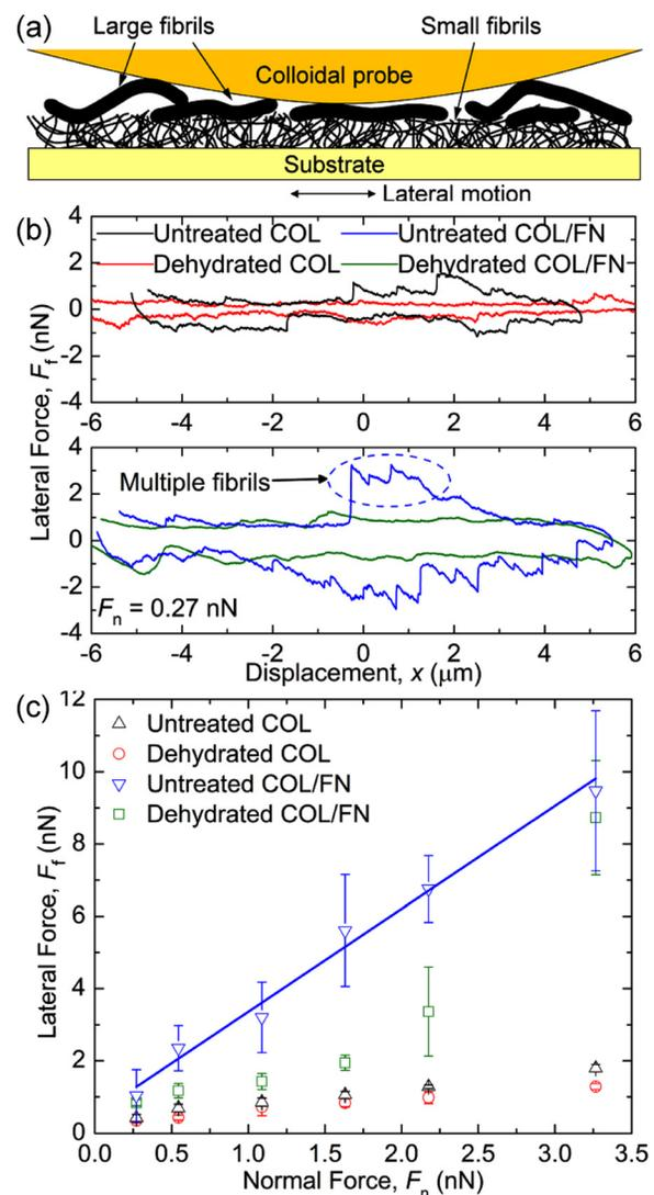
FIG. 2. (a) Schematic diagram of a colloidal probe in contact with a COL film.  $F_f$  as a function of (b)  $x$  and (c)  $F_n$  for the untreated and dehydrated COL films with and without FN. In (b), smooth sliding and stick-slip behavior with multiple instabilities are observed. In (c),  $F_f$  varies linearly with  $F_n$  for all films; the solid line represents a linear fit to the untreated COL/FN data, with  $\mu$  as the slope.
