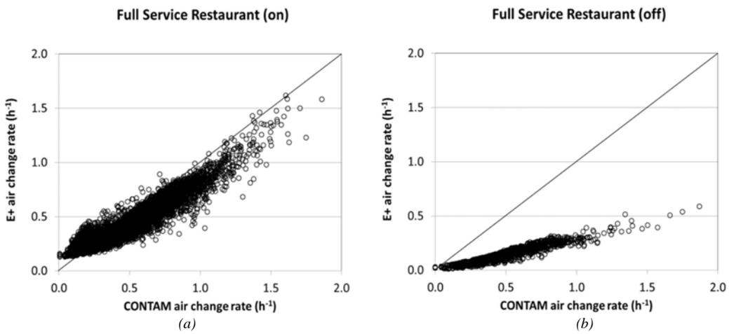
Figure 2. EnergyPlus vs. CONTAM infiltration rates for Full Service Restaurant (a) system-on and (b) system-off.
