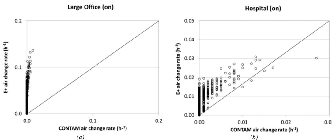
Figure 4. EnergyPlus vs. CONTAM infiltration rates for (a) Large Office system-on and (b) Hospital system-on, low  $I_{design}$  value ( $0.000304 \text{ m}^3/\text{s}\cdot\text{m}^2$ ).
