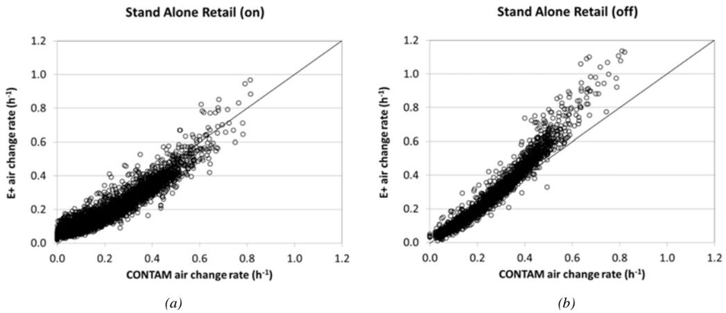
Figure 1. EnergyPlus vs. CONTAM infiltration rates for Stand Alone Retail (a) system-on and (b) system-off.
