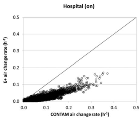
Figure 3. EnergyPlus vs. CONTAM infiltration rates for Hospital system-on.
