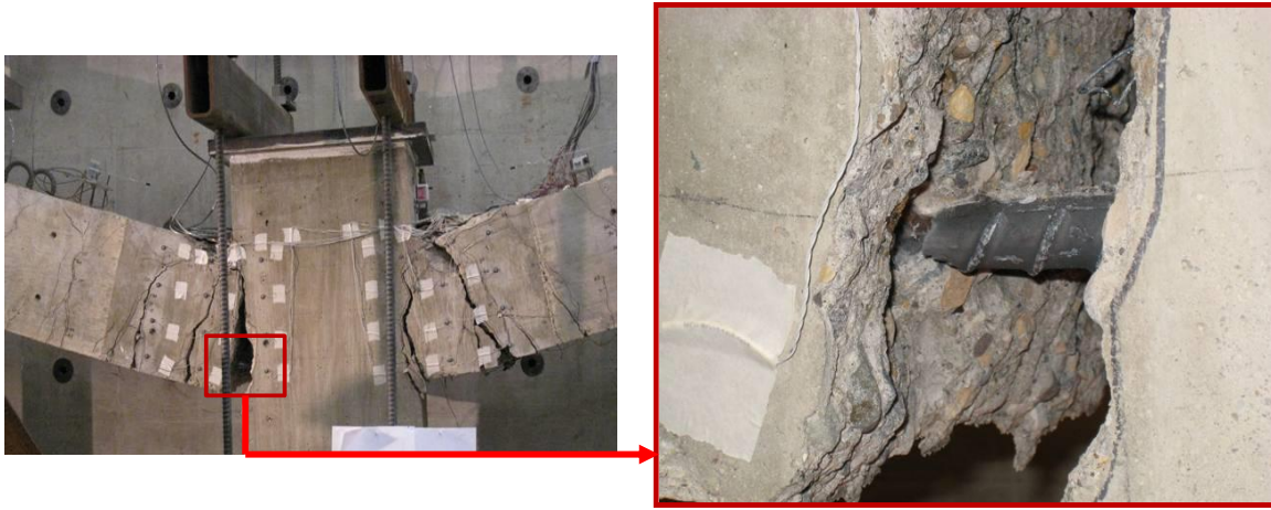
Figure 12: Failure mode of the reinforced concrete assembly.
