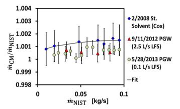
Figure 7. Comparison of the calibration of a 0.6 cm-diameter Coriolis meter in Stoddard solvent and 5 % PG + W mixture. The error bars are the expanded uncertainty (k = 2 corresponding to a 95 % confidence level) that accounts for uncertainties from: (1) the LFS, (2) the measured density and, (3) the reproducibility of the coriolis meter.
