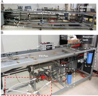
Figure 2. A) The 2.5 L/s LFS. B) The 0.1 L/s LFS. The plumbing that was replaced is outlined in red. The filters that were added are outlined in white.
