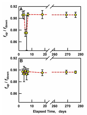
Figure 4. The ratio of the upstream rotor frequency to the downstream rotor frequency during 8 calibrations spanning almost a year. A) Turbine meter that was rinsed and dried in between each calibration. B) Turbine meter that was left continuously in reverse osmosis water. The error bars shown are the standard deviation of 7 measurements.
