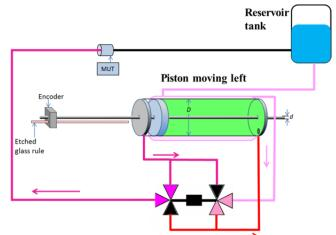
Figure 1. Sketch of the piston prover with the piston stroking left.
