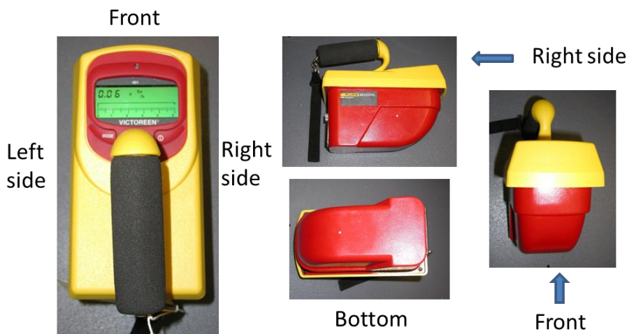
Figure 2: Shown are the reference points of the Victoreen® 451P and orientations
