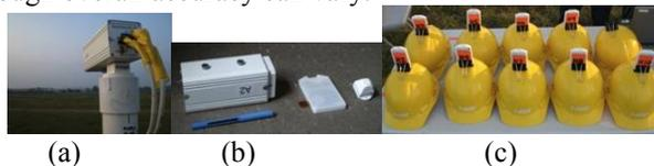
Figure 1. (a) Shows a UWB receiver deployed in the field (b) shows the asset tracking system components, ultra-wideband radio frequency receiver (shown with integrated
