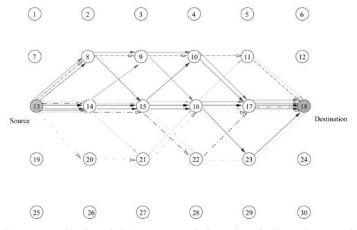
**Fig. 2** Grid wireless sensor network employing the CDSR routing protocol, where Node<sub>13</sub> and Node<sub>18</sub> are the source and destination nodes, respectively
