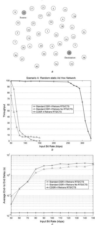
**Fig. 8** Scenario A: random static wireless sensor network The proposed CDSR scheme is capable of attaining a better performance than the standard DSR, not only in throughput but also in average end-to-end delay
