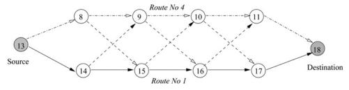
**Fig. 3** Distinctive routes that can assist the transmission of each other, which are selected using the proposed CDSR protocol for the wireless sensor network example of Fig. 2
