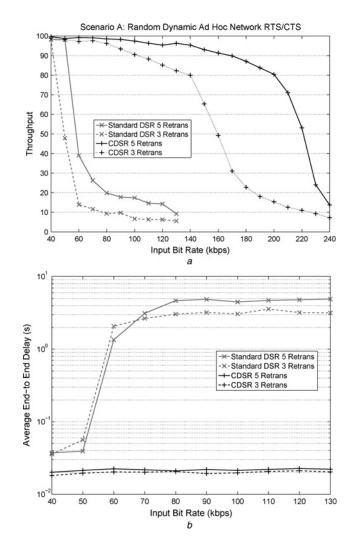
**Fig. 9** Scenario A: comparing the performance of the standard DSR with the proposed CDSR scheme based on a random dynamic wireless sensor network that is robust in resisting network topology variation caused by nodes' mobility
