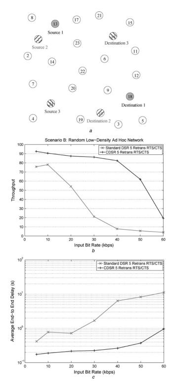
**Fig. 10** Scenario B: a multi-session scenario in a low-density wireless sensor network The proposed CDSR scheme is capable of achieving partial cooperative diversity and improving the performance
