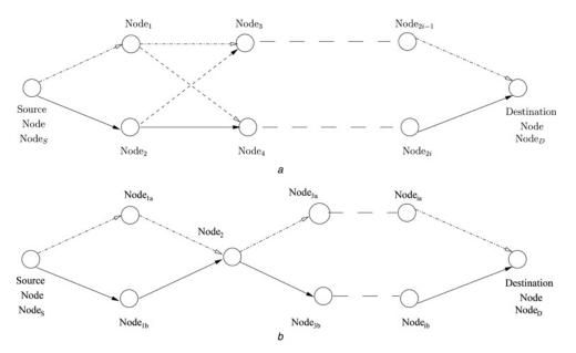
**Fig. 1** Solutions of the proposed cooperative multi-hop transmission scheme, which is selected by CDSR protocol of Section 3, scheduled by the cooperative MAC protocol of Section 4 and transmitted using TR-STBC of Section 5
