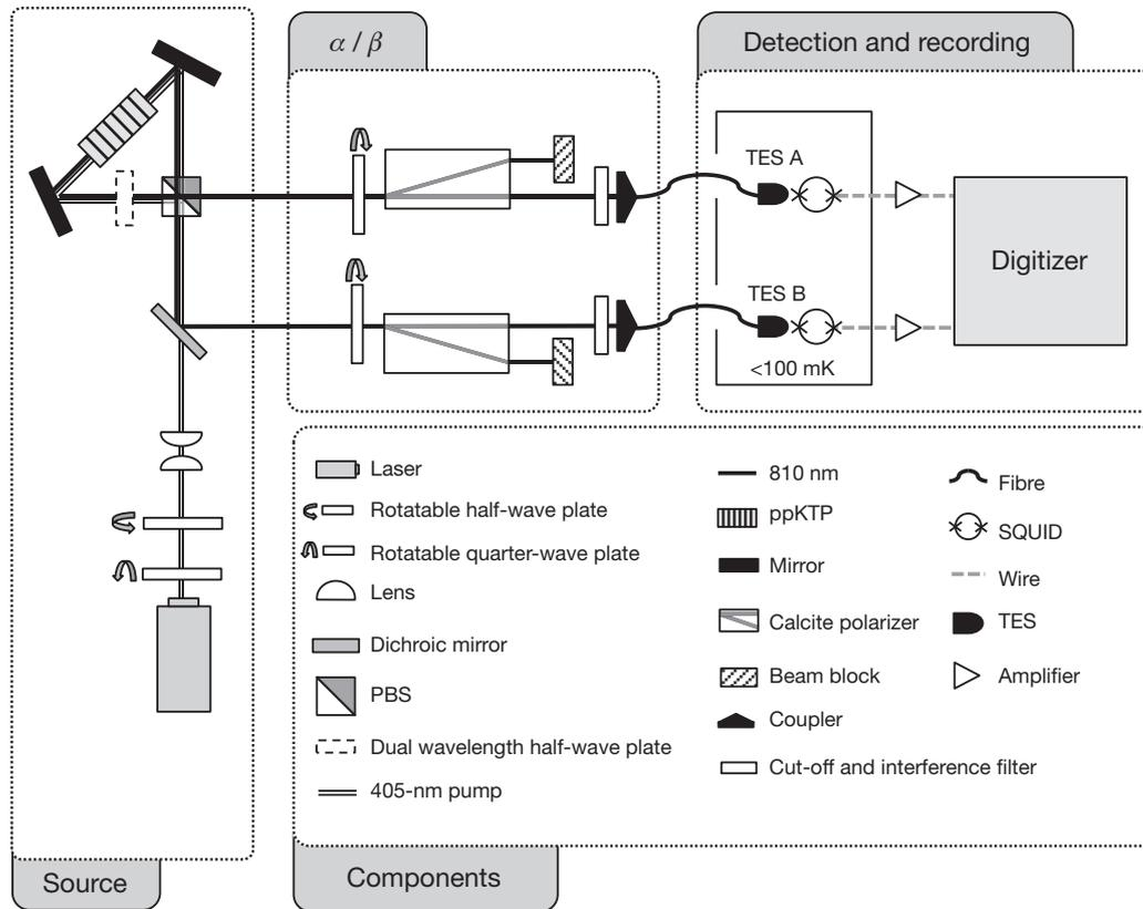
**Figure 2 | Measurement set-up.** The source, based on spontaneous parametric down-conversion in ppKTP (periodically poled potassium titanyl phosphate) in a Sagnac configuration, produces polarization-entangled photons with a wavelength of 810 nm. A measurement setting is implemented in each arm by rotating a half-wave plate to the desired angle in front of a calcite polarizer.
