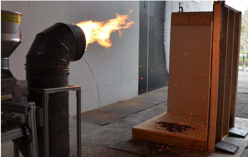
Fig. 6 Typical experiment exposing a decking assembly to continuous wind-driven firebrand showers. In this particular experiment, Cedar was used as the decking material.
