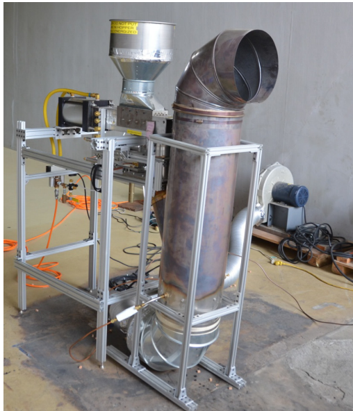
Fig. 2 Full-scale Continuous Feed Firebrand Generator installed in BRI's FRWTF. The device was not producing firebrands at the time of this photograph.
