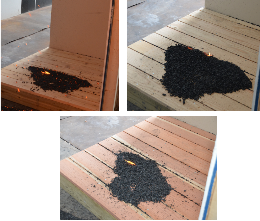
Fig. 7 Flaming ignition of Cedar, Douglas-fir, and Redwood decking assemblies.
