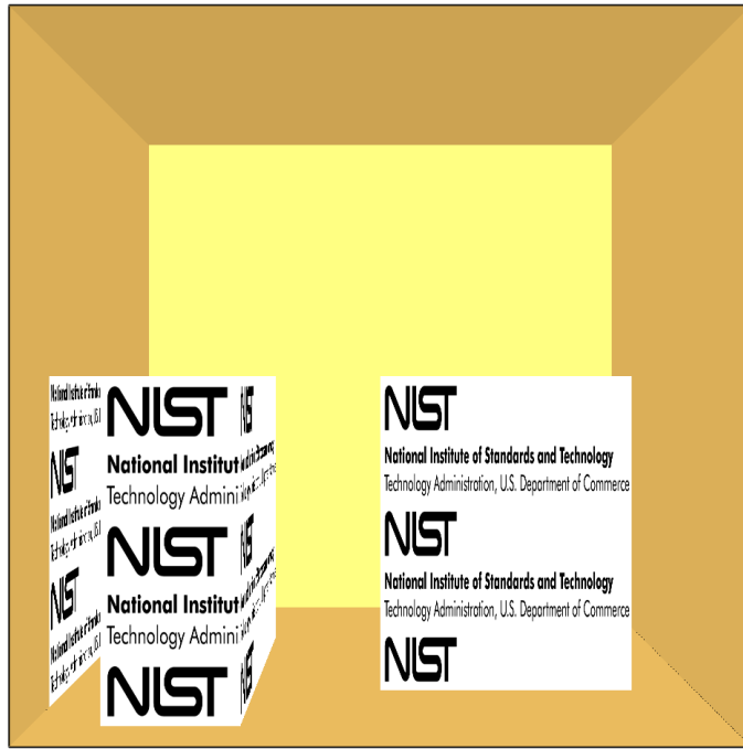
Figure 12.1: Texture map example. The same texture was applied to two different blockages and a vent (with different widths) by assigning different TEXTURE_WIDTH parameters in the input file.
