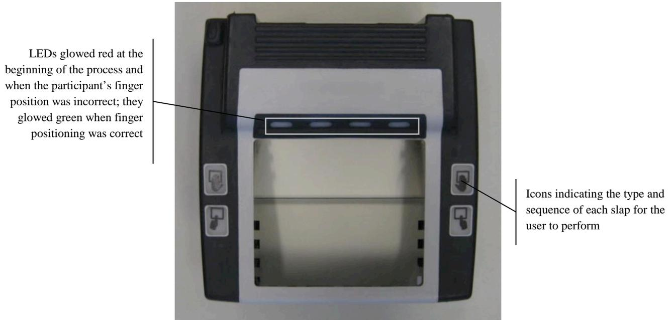
**Figure 3: Fingerprint scanner with indicators**
