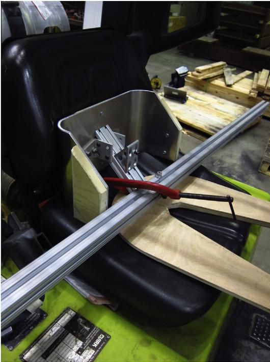
Fig. 8. The NIST-built, SIP fixture in place and loaded with weights.
