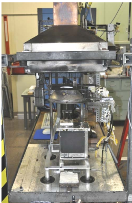
Figure 1. Modified Cone Calorimeter
