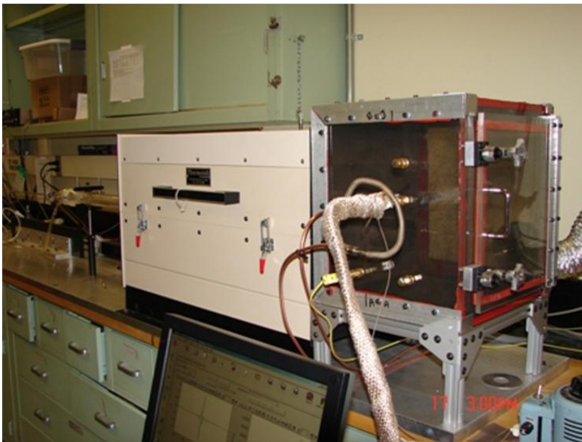
Figure 3. Closeup of the Sampling and Dilution Chamber
