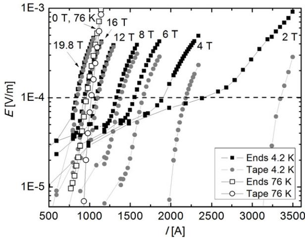
**Figure 8.**  $E$ - $I$  characteristics of cable CORC-2 as a function of magnetic field at 4.2 K, determined with two sets of voltage contacts; one set was located on the copper terminal (squares) and one set was located on one of the tapes in the outer layer of the cable (circles). Data taken at 76 K in self-field are included in the figure (open symbols). The dashed line indicates the electric field criterion of  $1 \mu\text{V cm}^{-1}$ .
