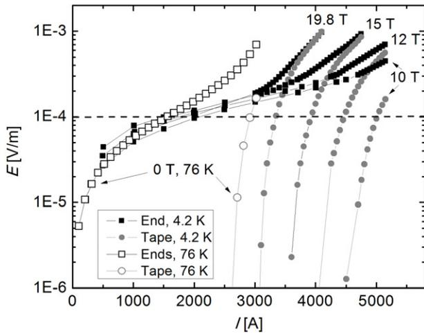
**Figure 11.**  $E$ - $I$  characteristics for cable CORC-3 at 76 K in self-field and at 4.2 K for magnetic fields ranging from 10 to 19.8 T. One set of voltage contacts was located on the copper terminal (squares) and one set was located on one of the tapes in the outer layer of the cable (circles). The dashed line indicates the electric field criterion of  $1 \mu\text{V cm}^{-1}$ .
