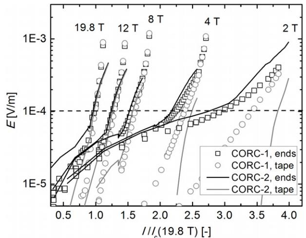
**Figure 10.** Electric field as a function of normalized current of cables CORC-1 and CORC-2 at different magnetic fields at 4.2 K. The applied currents are normalized to their cable  $I_c$  values at an applied field of 19.8 T to allow a direct comparison between the two cables that have different overall critical currents. The dashed line indicates the electric field criterion of  $1 \mu\text{V cm}^{-1}$ .
