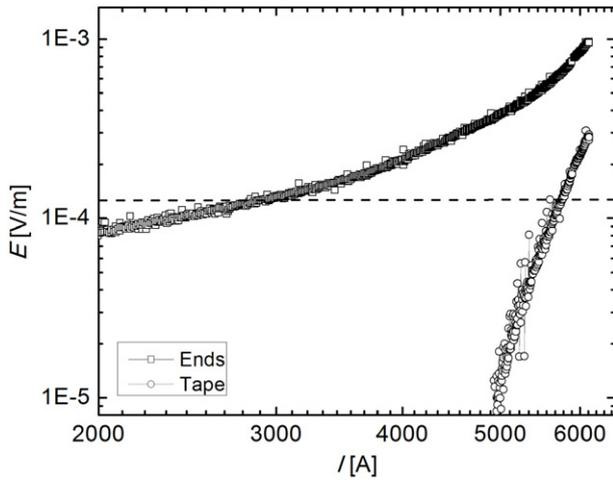
**Figure 13.**  $E$ - $I$  characteristics for cable CORC-4 at 4.2 K and a magnetic field of 19 T. One set of voltage contacts was located on the copper terminal (squares) and one set was located on one of the tapes in the outer layer of the cable (circles). The dashed line indicates the electric field criterion of  $1 \mu\text{V cm}^{-1}$ .
