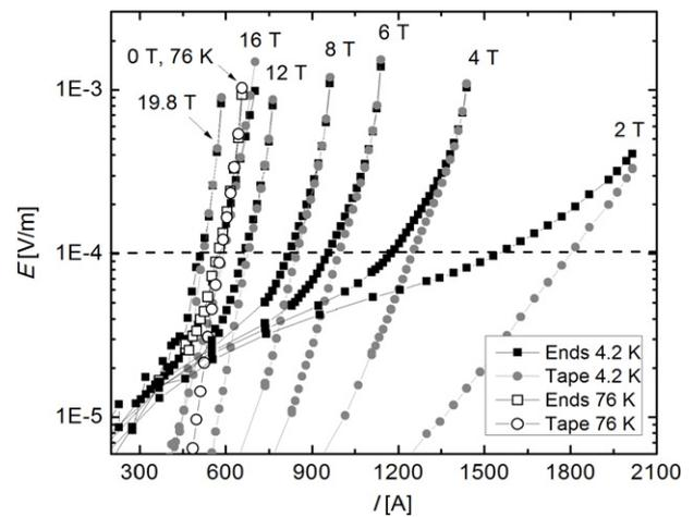
**Figure 4.**  $E$ - $I$  characteristics of cable CORC-1, measured with two sets of voltage contacts as a function of magnetic field at 4.2 K. One set was located on the copper terminal (squares) and one set was located on one of the tapes in the outer layer of the cable (circles). Included in the figure are the  $E$ - $I$  curves that were measured at 76 K in self-field (open symbols). The dashed line indicates the electric field criterion of  $1 \mu\text{V cm}^{-1}$ .
