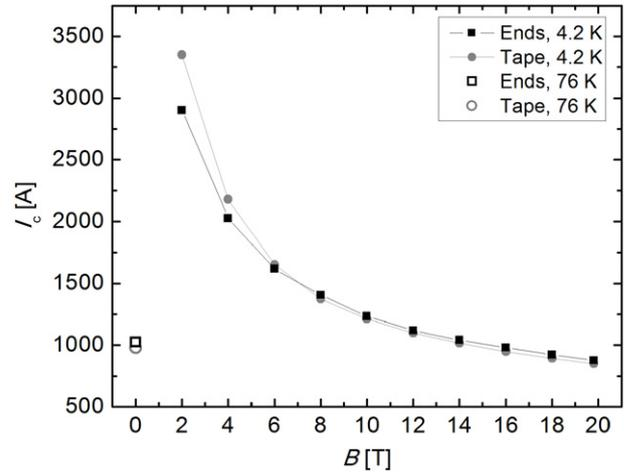
**Figure 9.** Magnetic field dependence of  $I_c$  of cable CORC-2 as determined with two sets of voltage contacts. Included in the figure are the critical currents of the cable at 76 K in self-field (open symbols).
