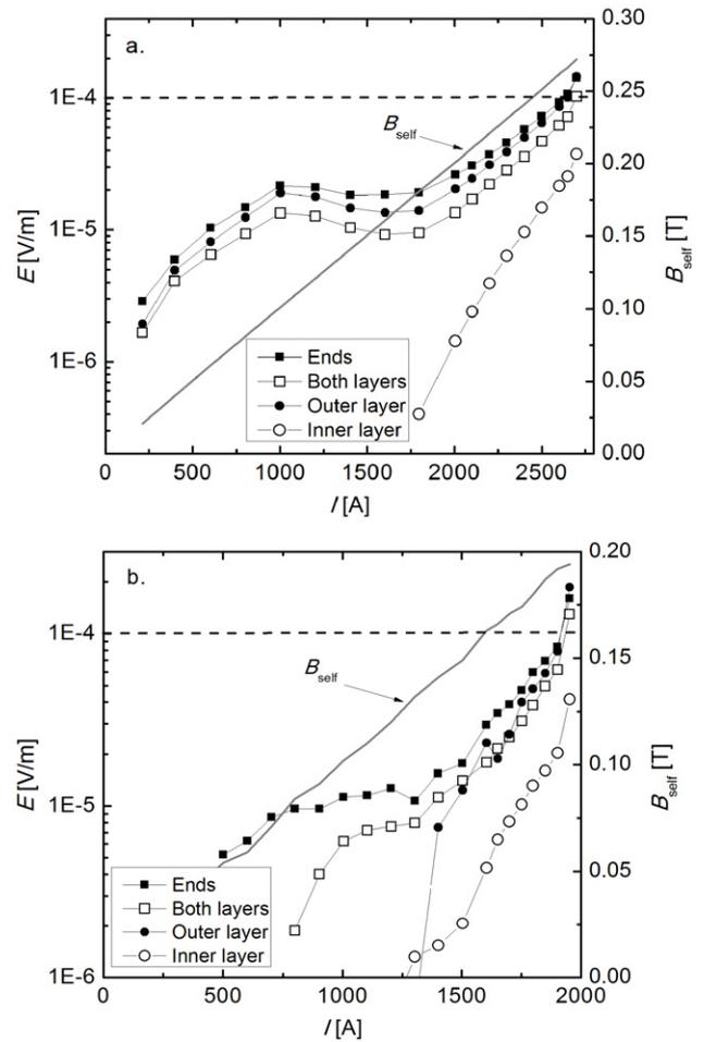
**Figure 14.** (a)  $E$ - $I$  characteristics of the magnet wound from cable CORC-5 at 4.2 K in a background field of 12 T. (b)  $E$ - $I$  characteristics at 4.2 K in a background field of 19.8 T. Four sets of voltage contacts were used in the measurements, as indicated in the figure. Included in both figures is the measured magnetic field generated by the coil. The dashed line indicates the electric field criterion of  $1 \mu\text{V cm}^{-1}$ .
