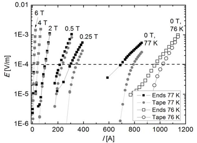
**Figure 7.**  $E$ - $I$  characteristics of cable CORC-2, as measured with two sets of voltage contacts. One set was located on the copper terminal (squares) and one set was located on one of the tapes in the outer layer of the cable (circles). All data were measured at 77 K, except for the two curves that were measured at 76 K in self-field (open symbols). The dashed line indicates the electric field criterion of  $1 \mu\text{V cm}^{-1}$ .
