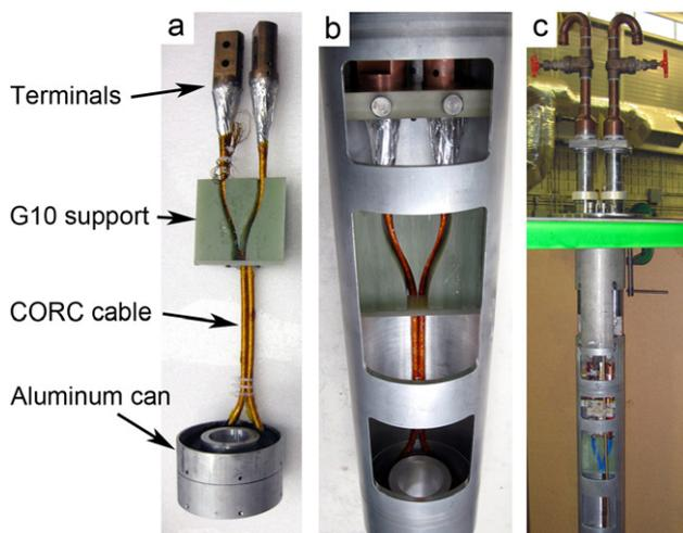
**Figure 3.** (a) CORC cable with local reinforcement provided by the epoxy-filled aluminum cup and the G-10 structure near the cable ends. (b) Cable inserted into the lower part of the support structure. (c) Magnet insert containing the cable sample and vapor-cooled current leads.
