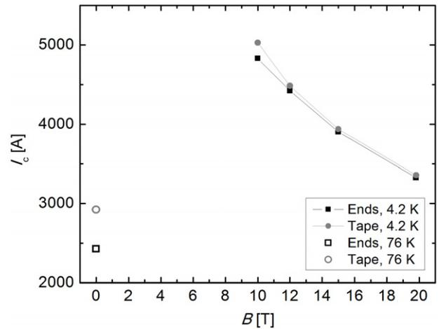
**Figure 12.** Magnetic field dependence of  $I_c$  of cable CORC-3 at 4.2 K, determined with two sets of voltage contacts. One set was located on the copper terminal (squares) and one set was located on one of the tapes in the outer layer of the cable (circles). The cable  $I_c$ s at 76 K in self-field are included (open symbols).
