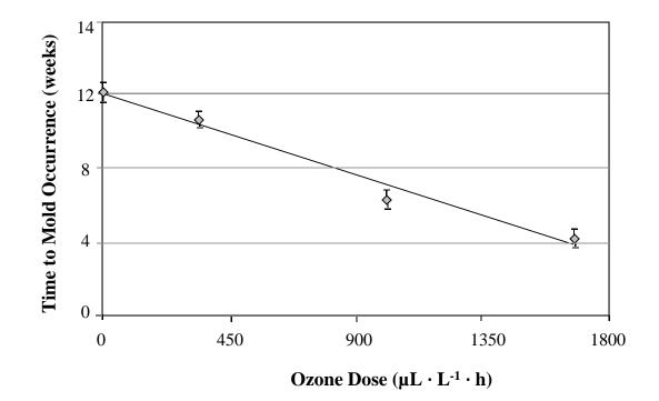
Figure 5. Effects of ozone dose on time to mold occurrence for ozone-treated bamboo incubated at 85 % RH and 30 °C condition. The error bars represent one standard deviation.
