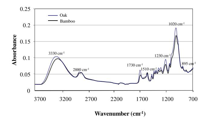
Figure 3. ATR-FTIR spectra of untreated bamboo and untreated oak.
