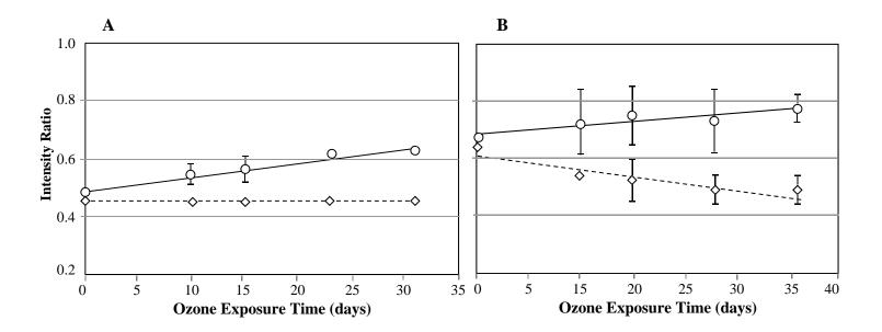
Figure 4. ATR-FTIR Intensity changes of the 1510 cm<sup>-1</sup> (◊) and 1730 cm<sup>-1</sup> (◊) bands as a function of ozone exposure for oak (A) and bamboo (B). The intensities have been normalized to that of the 895 cm<sup>-1</sup> band. The error bars represent one standard deviation.
