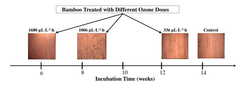
Figure 6. Representative optical microscopy images of entire-surface mold growth versus incubation time for untreated bamboo (control) and bamboo treated with ozone at different doses.
