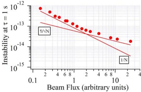
**Figure 4:** Measured instability at 1 second, as a function of beam flux. Data are shown as filled circles. The solid lines indicate  $N^{-1}$  and  $N^{-1/2}$  asymptotes ( $N$  scales with beam flux).
