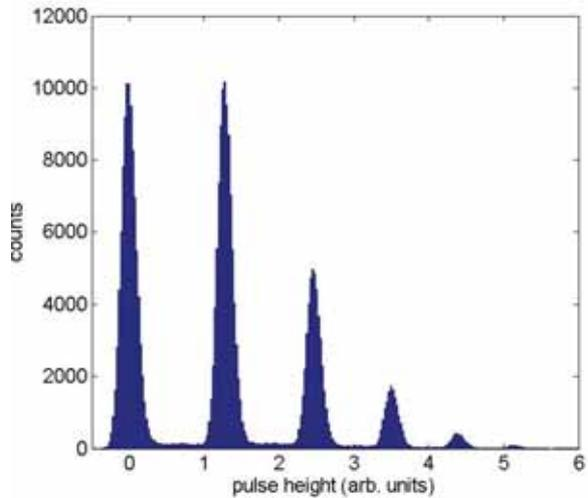
Figure 1: Photon pulse height distribution for a measured coherent state with a mean photon number of about 1.
