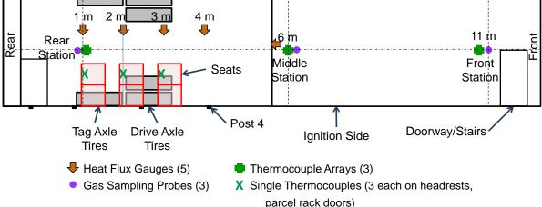
*Figure 6* (*Top*) *Photograph showing the assembly of the original motorcoach rear half and added front.* (*Bottom*) *Diagram showing the layout of measurements for the tenability test.*
