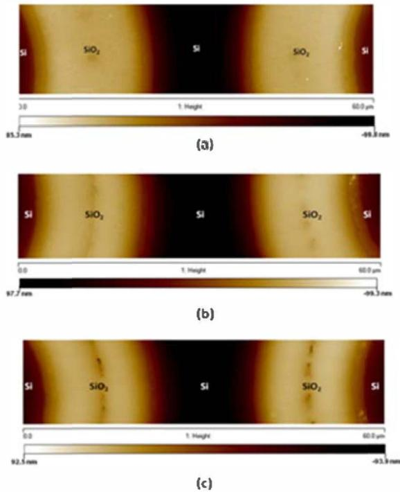
Figure 2: AFM topography image showing the morphological evolution of the SiO<sub>2</sub> isolation liner with thermal cycling. (a) As-received state (b) after 1000 thermal cycles (c) after 1600 thermal cycles.
