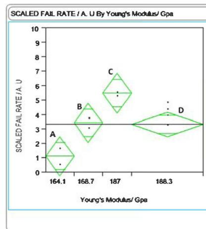
Figure 5: Correlation between post-packaging failure rates and the Young's modulus of various encapsulating dielectric types.
