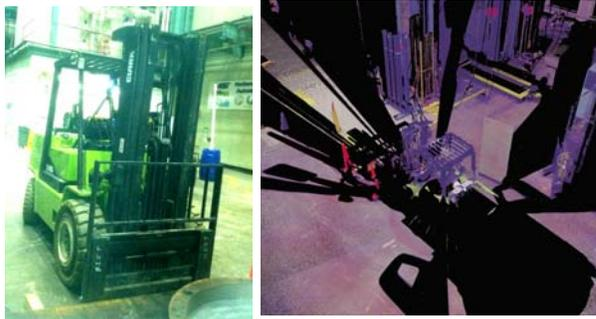
*Figure 18 – (left) forklift with scanner located at the operator's head location and (right) data plot from the scanner showing (black) occluded regions.*
