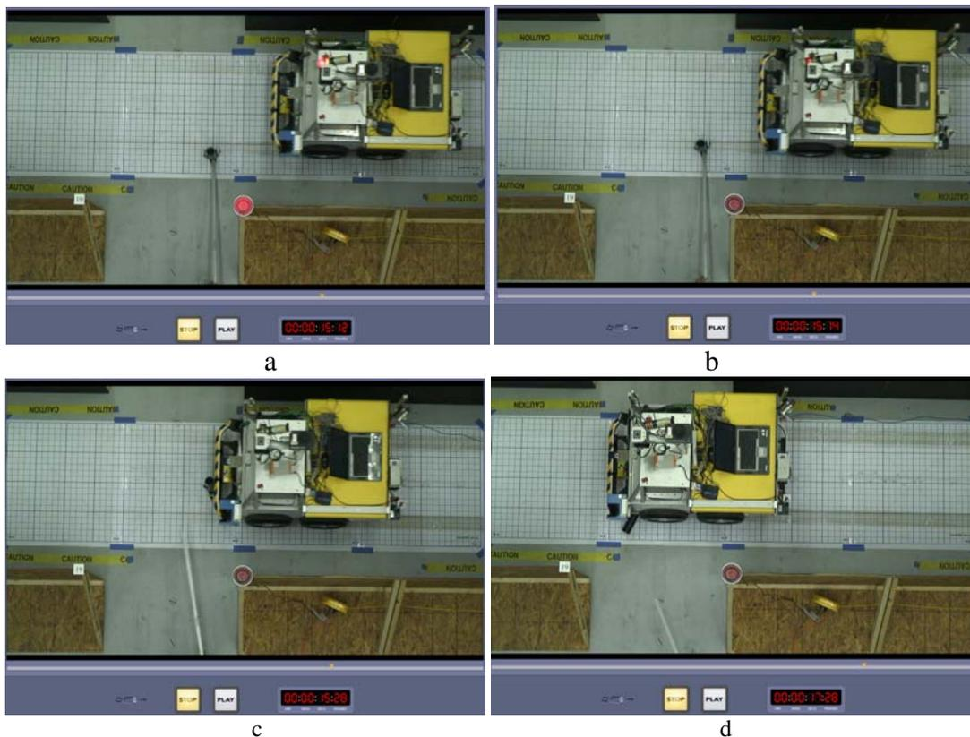
*Figure 5 – Snapshots from the overhead video showing when: (a) the test piece crosses the photo-sensor, (b) the test piece is detected by the AGV safety sensor, (c) the AGV hits the test piece (or when the test piece stops in the AGV path), (d) the AGV stops.*
