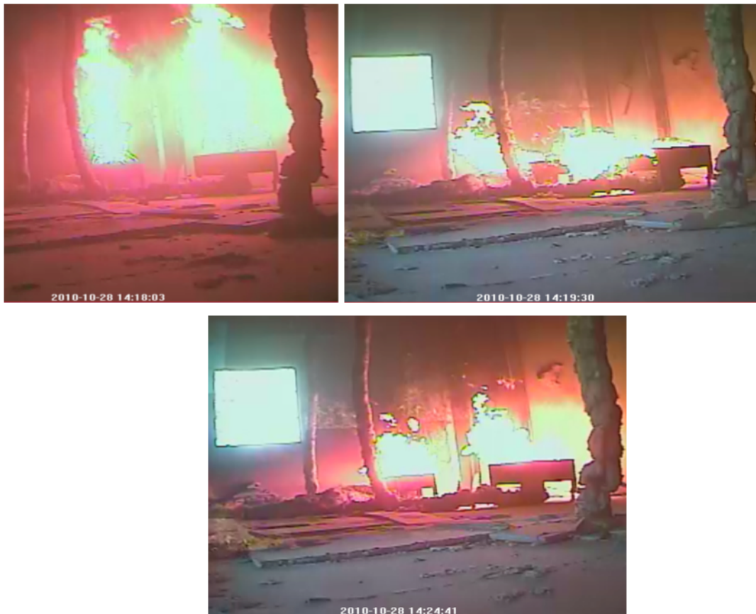
Figure 4.2.4: Still images from Open Vent PPV experiment. Top left: prior to ventilation. Top right: during PPV application. Bottom: PPV application during the time interval with increased wind speeds.
