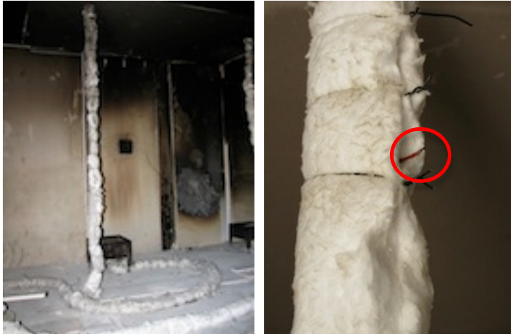
Figure 3.3.23: The image on the left shows a thermocouple tree with insulation with one of the two sand burners behind it. The image on the right shows a thermocouple protruding from the insulation, circled in red.
