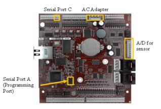
Figure 8 - Hardware setup for IEEE 1451.2 TIM
