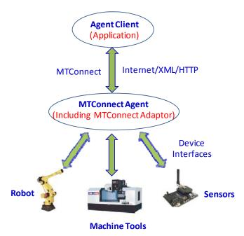
Figure 1 - Architecture of MTConnect
