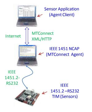
Figure 7 - Prototype integration system
